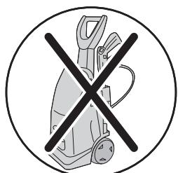
Luminaire must not be cleaned by means of high-pressure washer.
