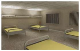
Scheme: 4-bed ward, 7.6m x 6.6m x 2.7m Luminaire(s) used: Bedhead mounted uplight and reading light Ward floor:  $E_{av} = 141$  lux ;  $E_{mv}/E_{av} = 0.68$
