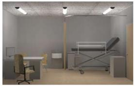
$\label{eq:scheme:consulting room, 8m x 3m x 2.7m} \mbox{Luminaire(s) used: 3 Diffusalux Hospital 2x35W T16} \mbox{Desk height: } E_{\alpha} = 440 \mbox{ lux ; } E_{min}/E_{\alpha} = 0.7 \mbox{}$
