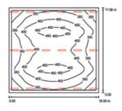
Scheme: Multi-purpose sports hall,  $17m \times 18m \times 7.6m$ Luminaire(s) used: 18 x Titus Sport 4 x 49W, 7.6m mounting height Floor:  $E_{av} = 364 |ux; E_{mv}/E_{av} = 0.61$
