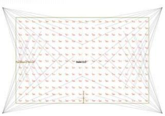
Scheme: Football stadium with 4 x 25m corner columns Luminaire(s) used: 48 x Mundial R 2kW HQFTS Pitch:  $E_{av}$  = 538 lux;  $E_{min}/E_{av}$  = 0.76
