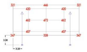
$\label{eq:scheme: Double tennis court, 24m x 11m} \mbox{Luminaire(s) used: 4 x Champion 2kW HQI-TS/N/L, 12m mounting height Pitch: $E_{ov}$ = 397 lux, $E_{mer}/E_{ov}$ = 0.81 $\end{tabular}$
