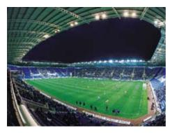
A football stadium lit using Mundial floodlights. The luminaires are mounted along the roof of the stand down two sides of the pitch, and a mix of light distributions is used to correctly illuminate all the playing area. Lighting levels for television are supplied by ensuring good levels of vertical illumination in the camera directions.
