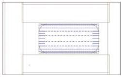
$\label{eq:scheme:licehockey stadium, 117.5m x 17.3m x 23m \\ \mbox{Luminaire(s) used: } 316 x \mbox{ Indus XS, } 2 x 80WT16, 17m mounting height \\ \mbox{Pitch: } E_{av} = 422 \mbox{ lux ; } E_{aw}/E_{av} = 0.07 \\ \end{tabular}$
