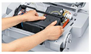
**Step 3:** Open the gear housing cover to access the connectors for main supply and controls.
