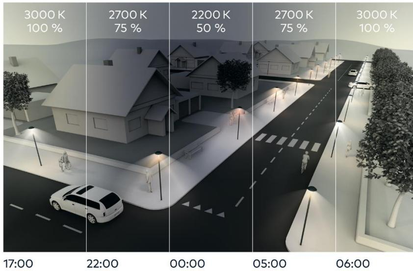
NightTune works by mixing light from warm and cool LEDs. By dimming the two groups of LEDs up and down separately, colour temperatures ranging from a warm 2200K to a moderate 3000K can be achieved, at different levels of brightness.
