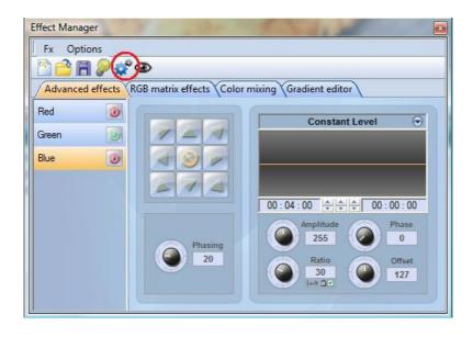
The Effect Manager adapts it's self depending on the fixtures you are using. To demonstrate the capabilities this tool, we'll start by using a matrix of generic RGB LED colour mixing fixtures.
